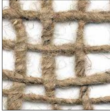
Jute mulch control netting
