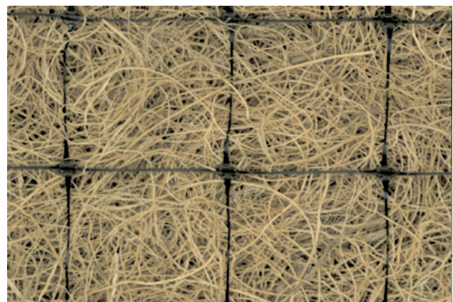
Close-up of extruded plastic netting
