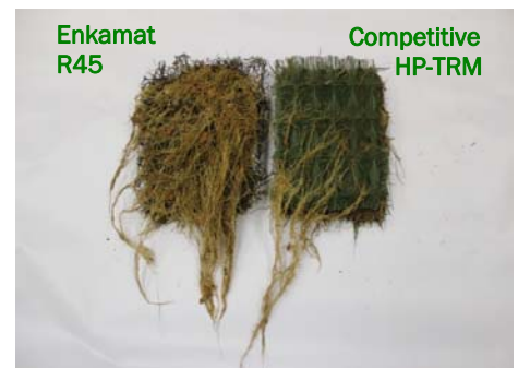
Washed specimens showing relative root development
